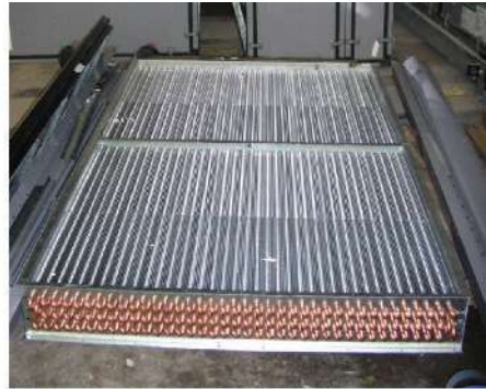
Figura 65 Serpentina de Aire Acondicionado.< https://www.google.com.mx/search > Consultada 1/Feb/2016
