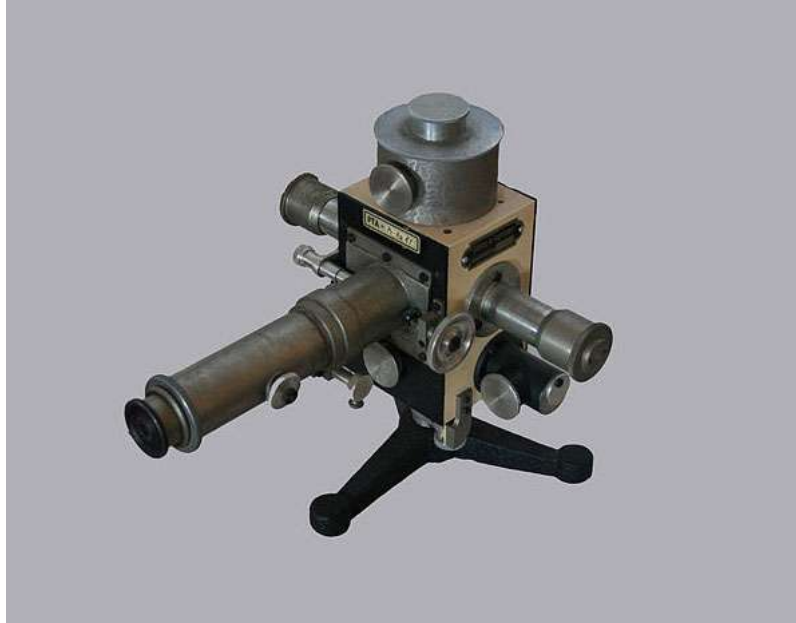
Figure 1.4: Wulf's electroscope. The instrument mainly consisted on a pair of quartz fibbers attached at the bottom to a bend quartz fibber. The distance of the two fibbers is measured through a microscope. The company Günther & Tegetmeyer was in charge of manufacturing Wulf's electroscopes [10]. Image source: https://commons.wikimedia.org/wiki/File:Originalwulf.jpeg .
