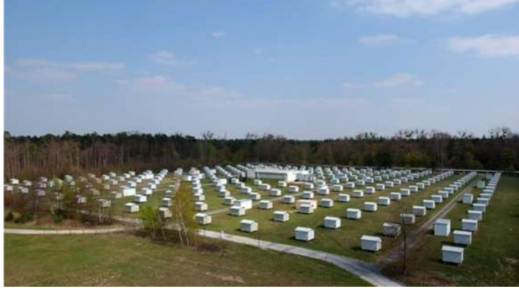
Figure 3.4: The KASCADE experiment was located at 110 m above sea level (1022 g/cm 2 ). The central detector of KASCADE was located at the big central building of the image, it was surrounded by a rectangular array of 252 scintillation detector stations. The stations were distributed over an area of 200 × 200 m 2 , and were equally spaced by 13 m [117].
