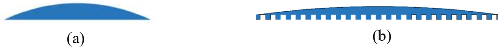
Figure 3.3.5. Wetting state on smooth surface (a) and rough surface (b) with hydrophilic materials (Wenzel model).
