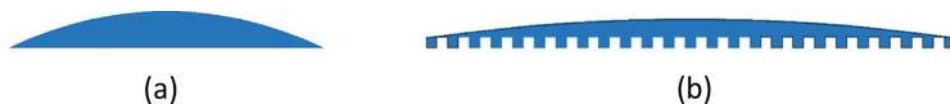
Fig. 6. Wetting state on smooth surface (a) and rough surface (b) of a hydrophilic material (Wenzel model).
