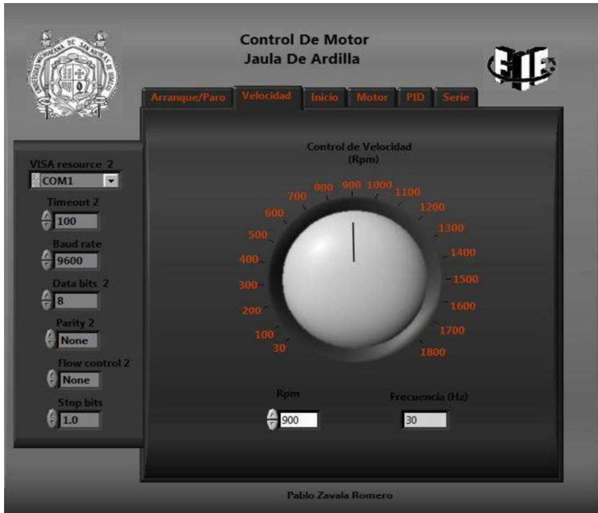
Figura 5.8 Panel Frontal del software de control.
