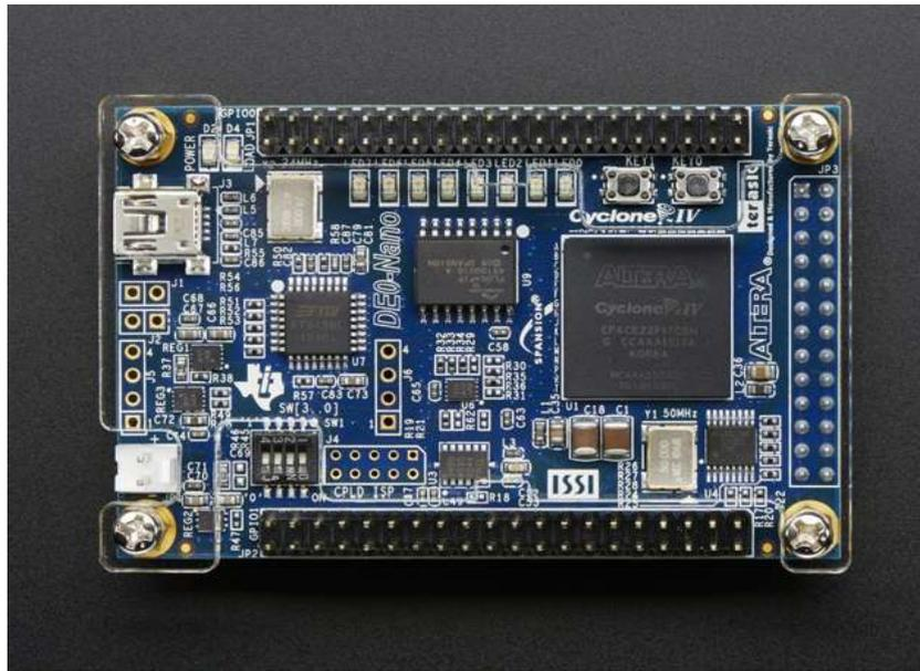
FIGURA 3.6: FPGA Cyclone IV EP4CE22F17C6N
