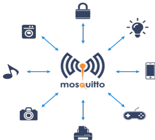
Figura 25: MQTT Broker, clientes MQTT, Mosquitto, fuente: [42]
