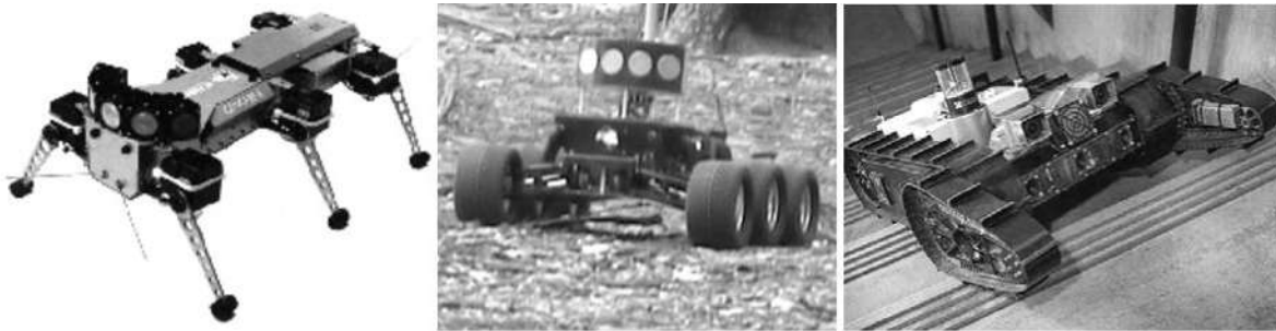
Figura 2-2 Robots terrestres. (a) Hermes (Robosoft). (b) Journey (SMU). (c) Scour (USF). [16]
