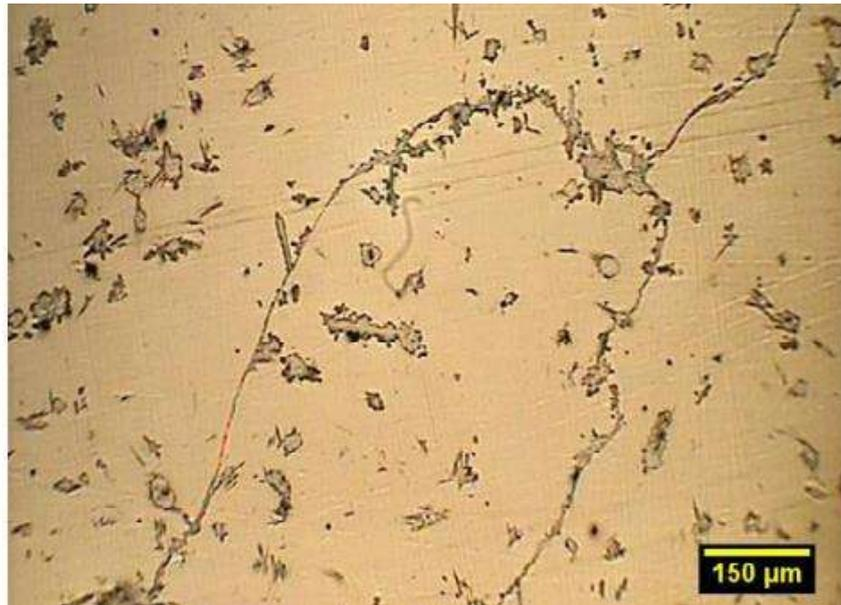
**Figura 2.5** Microestructura de un Acero Hadfield de composición 1.19% C, 0.476% Si, 12.4% Mn, 0.0317% P, 0.0084% S, 1.34% Cr, 0.0219% Mo, 84% Fe [51].
