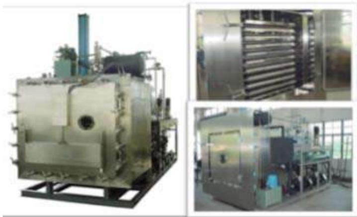
FIG 20: LA CÁMARA, ESTANTES, CONTROL DE VACÍO.
