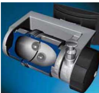
Figure A- 3: Oscillations in a horizontal position for balls and grinding jars.
