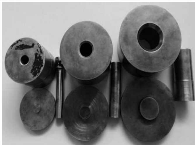
Figure 3- 2: Different die diameters 10, 15 and 25mm.
