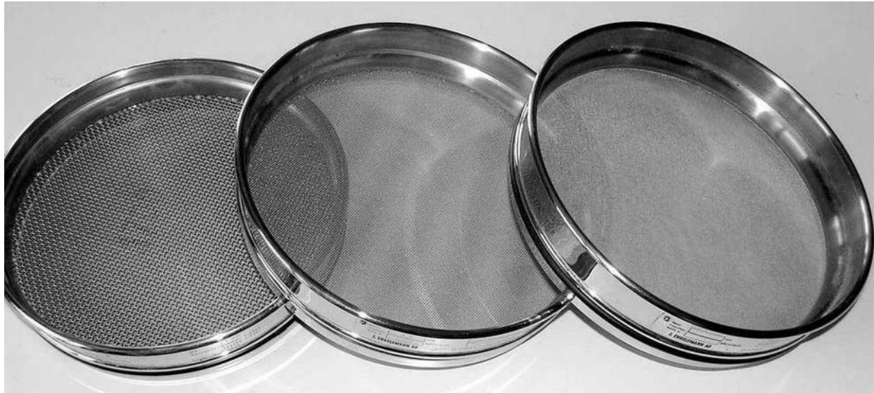
Figure A- 4: Different sieve holes sizes.
