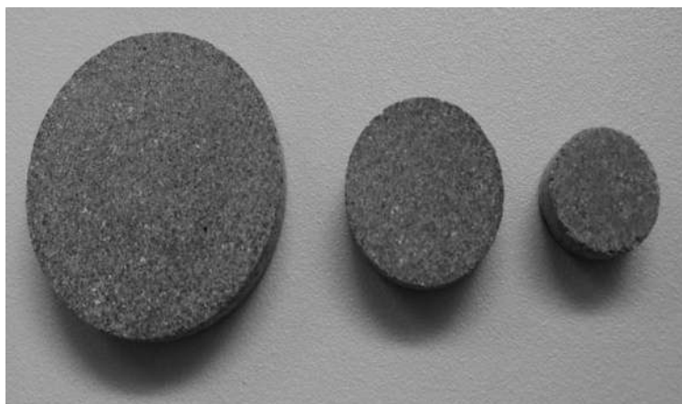
Figure 3- 3: Different pellet diameters 25, 15 and 10mm.
