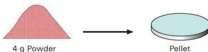
Figure A- 9: Procedure to make pellet without wax.
