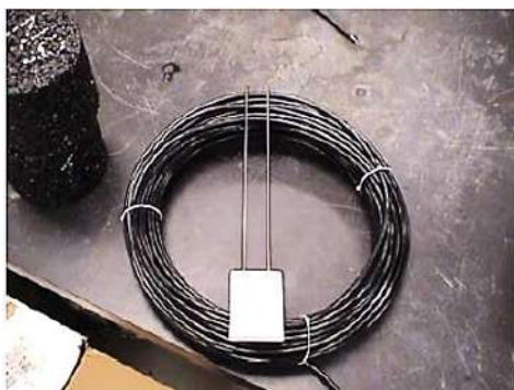
Figura 67 - TDR (Time Domain Reflectometry) (Timm, Priest, & McEwen, 2004).
