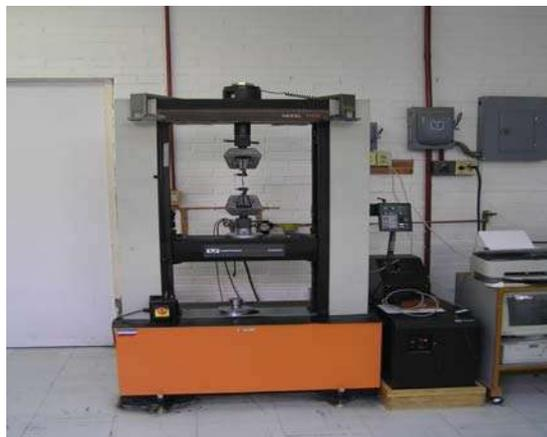
Figura 3.10 Máquina Universal INSTRON.
