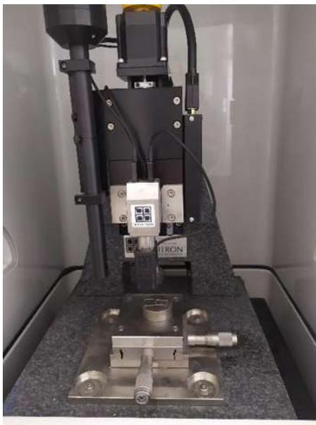
**Figura 3.15** Nanoindentador Hysitron Nanomechanical Test Instruments.
