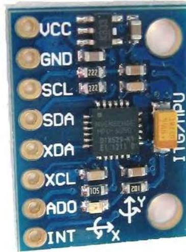
**Figura 44** Sensor MPU 6050
