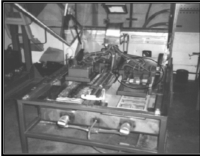
Figura 6.6 Máquina de ensayo, Purdue University Laboratory Wheel Tracking.
