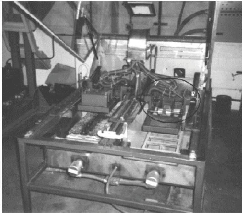
**Figura 5.4** Máquina de ensayo, Purdue University Laboratory Wheel Tracking (fuente: [www.asphaltwa](http://www.asphaltwa)).
