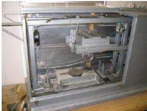
Figura 5.2 Georgia Loaded Wheel Tester (GLWT) (fuente: [www.asphaltwa.com](http://www.asphaltwa.com)).
