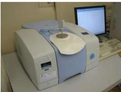
**Figura 6.** Perkin Elmer Spectrum 100 FT-IR
