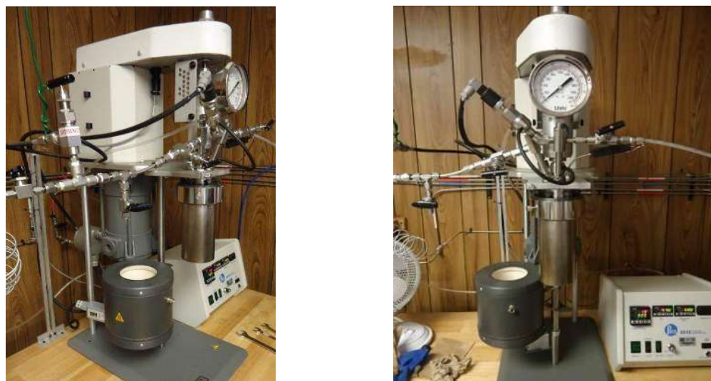
Figura 20.- Reactor batch Parr 4848
