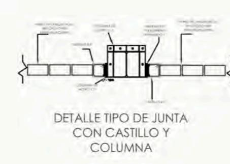
DETALLE TIPO DE JUNTA CON CASTILLO Y COLUMNA
