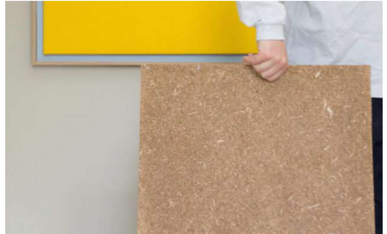
FIG.60 Tablero de compostaje
