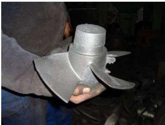
Figura 2.14 Micro-turbina Kaplan
