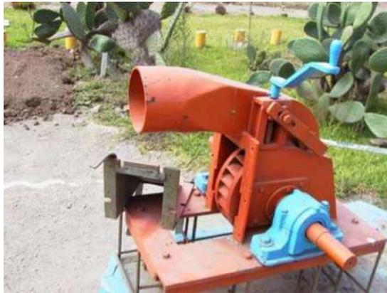
Figura 2.10 Micro-turbina Michell-Banki
