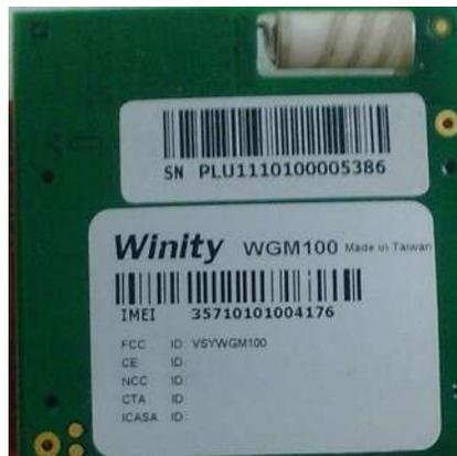
Figura 3: Modem GSM Winity modelo WGM100.
