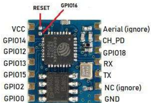
Figura 2.4.4-6 . ESP-04 pinout. [42]
