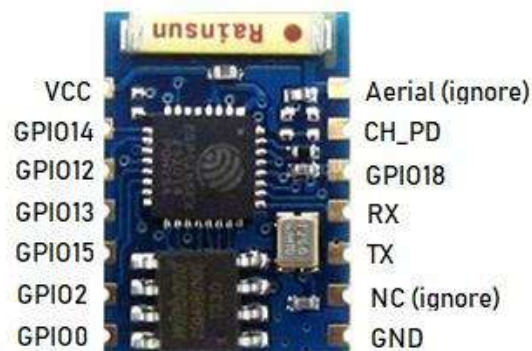
Figura 2.4.4-5 ESP-03 pinout [41]
