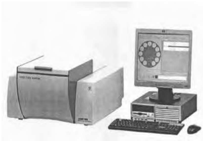
Figure 2.2: XRF device used to characterize the powder samples
