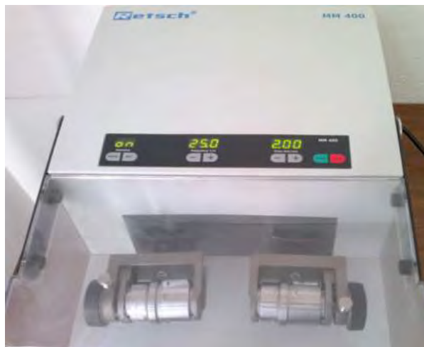
Figure 2.1: Milling machine to prepare the powder samples
