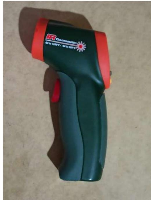
Figura 61: IR Thermometer 42510A.
