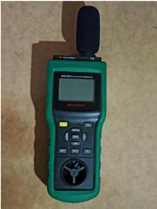
Figura 60: MS6300 Environment Mltimeter.
