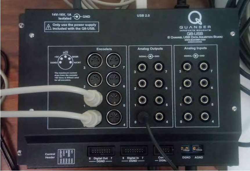
Figure 4.16: Quanser Q8-usb data acquisition device board
