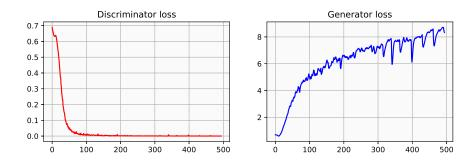
Figure 3.3: Convergence failure refers to not finding an equilibrium between the discriminator and the generator.
