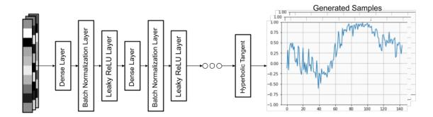
Figure 4.5: The generator receives a noise vector and transform it into a sequence that should have the same characteristics as the real samples.
