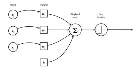
Figure 2.1: An example of the simple Perceptron network architecture that accepts a number of inputs, computes a weighted sum, and applies a step function to obtain the final outcome.
