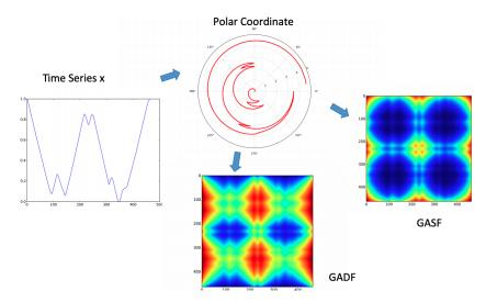
Figure 5.2: Encoding map of Gramian Angular Fields. [Wang and Oates, 2015] transformed a sequence into a polar coordinate system and calculate its Gramian Angular Summation/Difference Fields.
