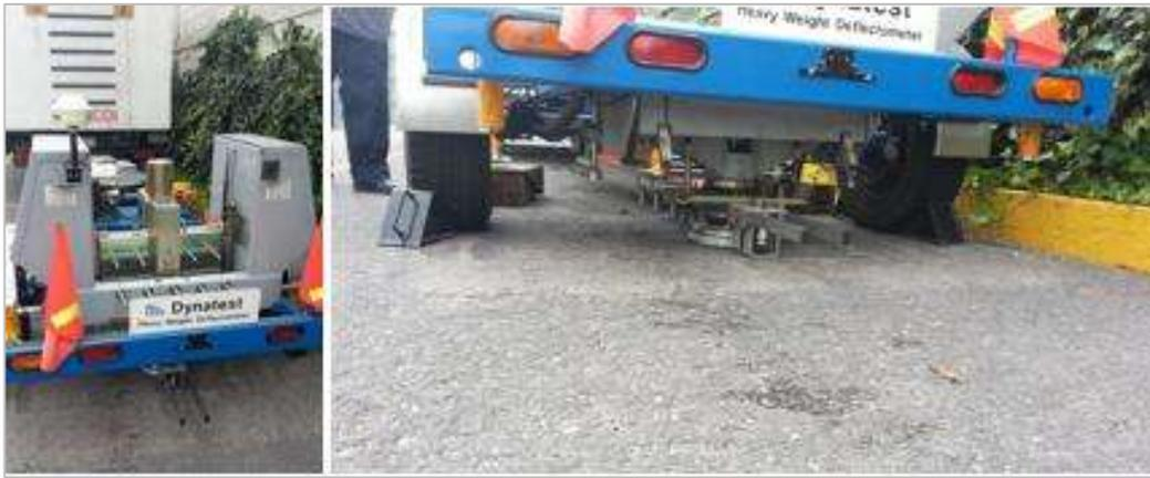
Figura 16.- Heavy Weight Deflectometer (HWD).
