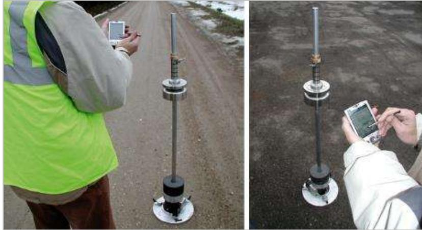
Figura 11.- Light Weight Deflectometer (IMT, 2014).
