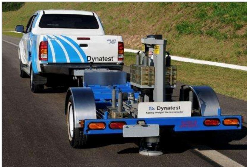
Figura 12.- FWD (Falling Weight Deflectometer).
