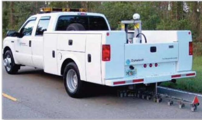
Figura 14.- Truck Mounted Deflectometer (TMD).
